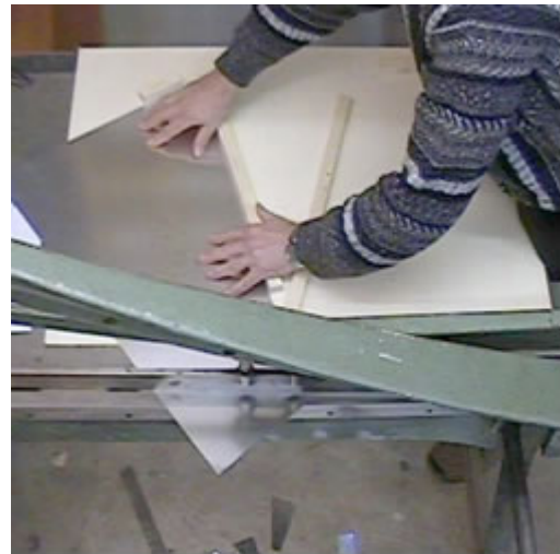
Fig. 15 The parts are cut with simple stops
