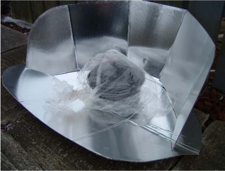
Figure 1: The CookKit with oven roasting bag. Note how the bag forms large air gaps around the pot.
