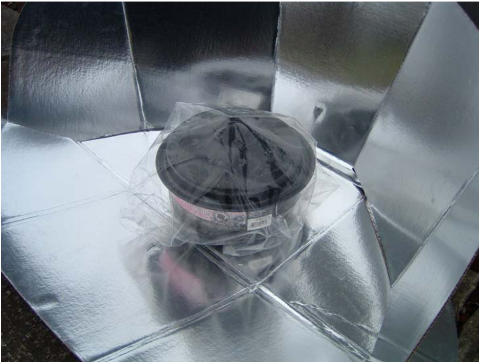
Figure 2: CookKit with 2-ft square sheet of PFA. The sheet is wrapped tightly around the pot, which forms smaller air gaps around the pot.
