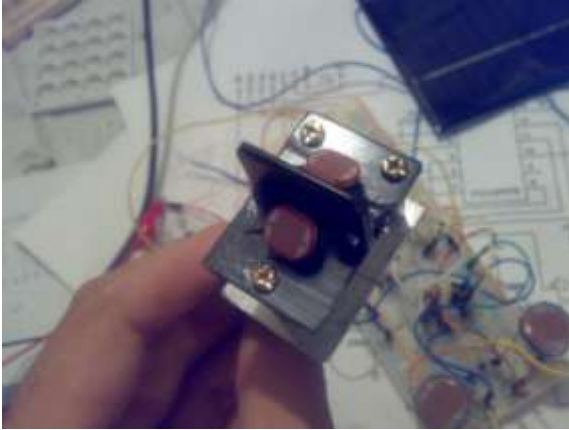
Fig. 3 : Traker sensor which I made it (two LDRs with a shade between them and adjustable mounting)
