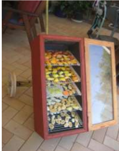
Solar fruit drier attached to golf buggy
