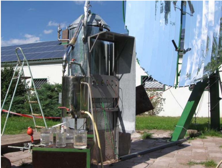
Fig. 2 Solar distillation system for essential oils extraction
