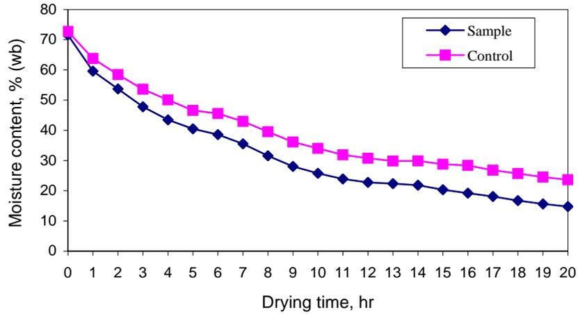
Fig. 20. Variations of moisture content with time for a typical experimental run during solar drying of silver jew fish
