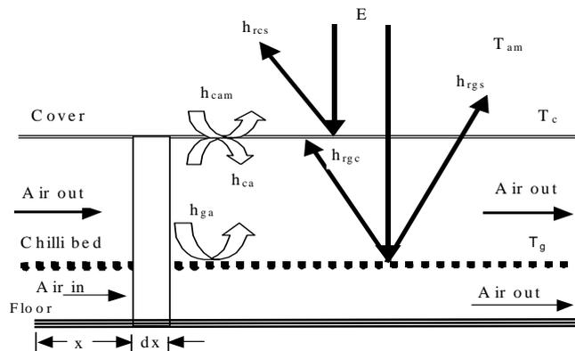
Fig. 10. Energy balances in the solar tunnel drier of depth, *b*
