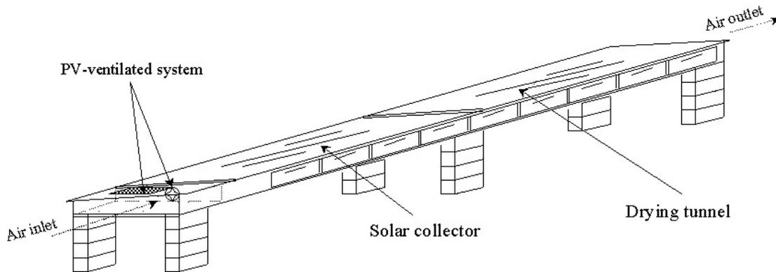
Fig. 5. Schematic diagram of the solar tunnel dryer with polycarbonate cover
