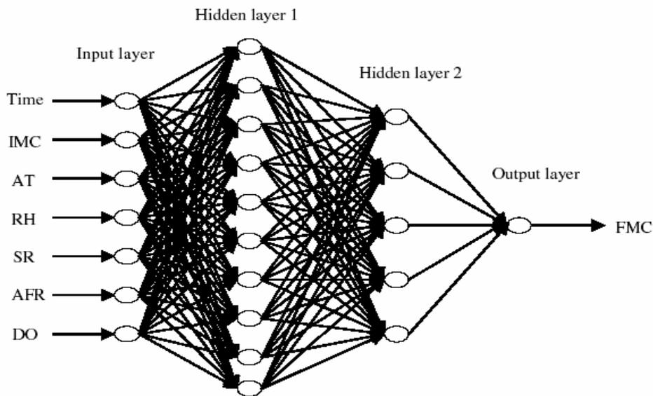
Fig. 11. The structure of the ANN solar tunnel dryer model for drying jackfruit bulb and jackfruit leather
