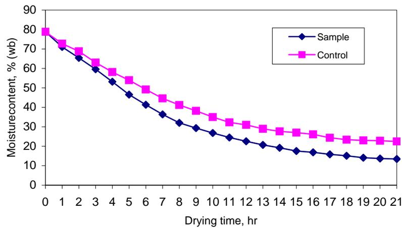
*Fig. 12. Variations of moisture content with time for a typical experimental run during solar drying of mango.*
