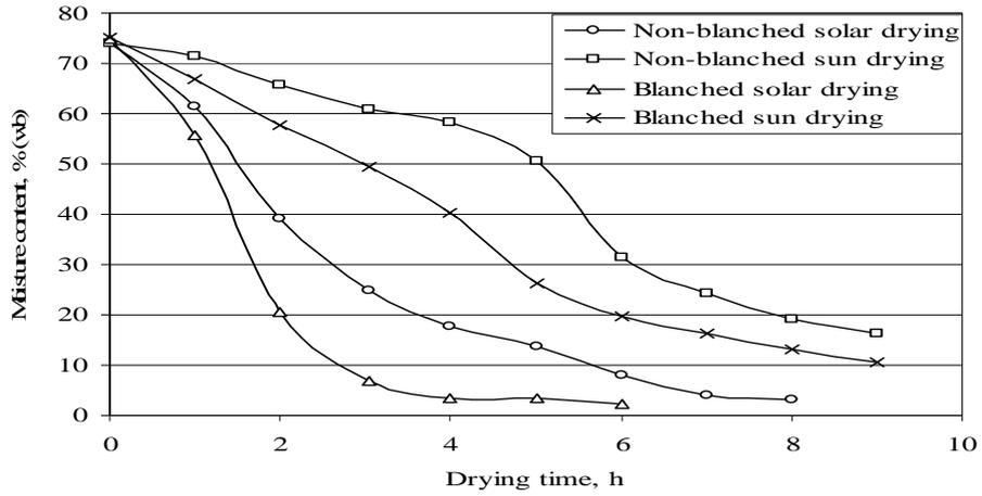
Fig. 18. Comparison of the moisture changes inside hybrid solar dryer and open sun drying during drying of Vasaka leaves
