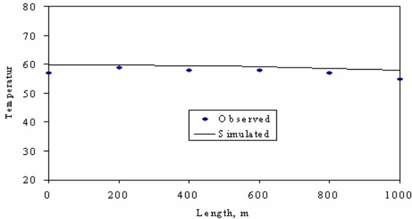
Fig. 21. Observed and simulated air temperature along the length of the dryer
