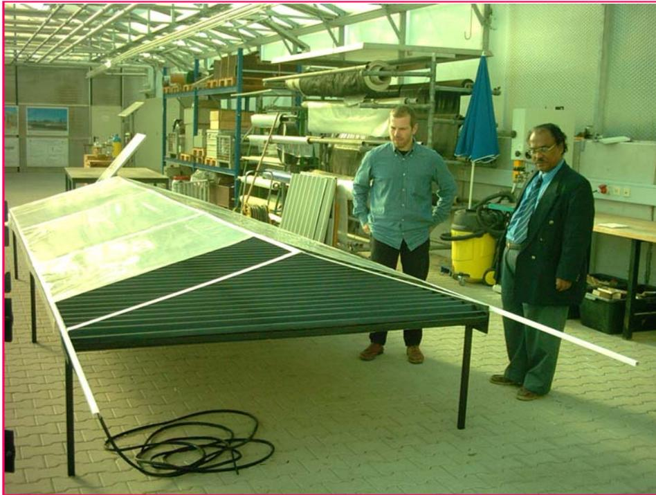
*Fig. 3. Pictorial view of the solar tunnel dryer under construction*
