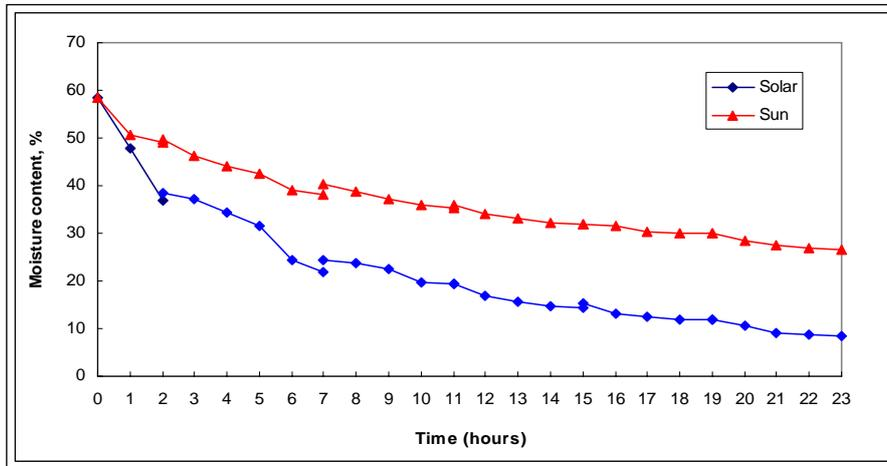
Fig.17. Variation of moisture content with time of day for a typical experimental run during solar drying of coffee.
