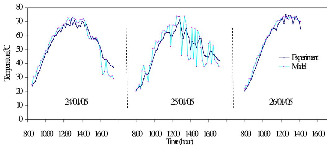
Fig. 23. Predicted and experimental values of the outlet temperature of the roof-integrated collector
