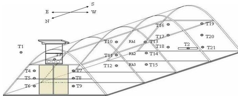
*Fig. 6. Schematic diagram of the greenhouse type solar dryer with polycarbonate sheet*
