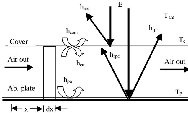
Fig.9. Heat balances in the flat plate solar collector of depth, *b*
