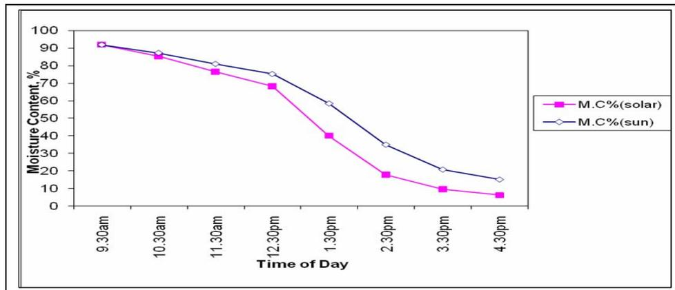
Fig. 14. Variations of moisture content with time for a typical experimental run during solar drying of mushroom.
