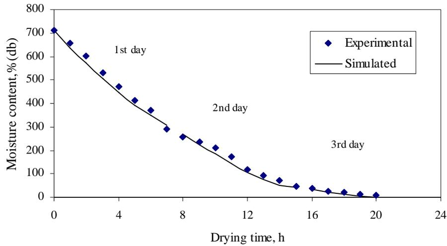
Fig. 22. Experimental and simulated moisture content at the outlet end of drier during drying of green chilli (After Hossain et al 2003)
