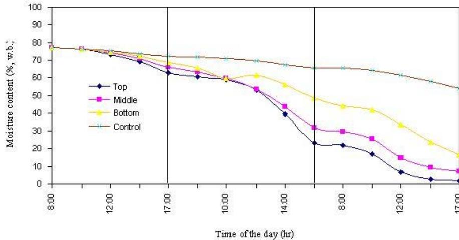
Fig. 15. Comparison of the moisture contents of chilli inside the greenhouse dryer with the traditional sun drying method for a typical experimental run.
