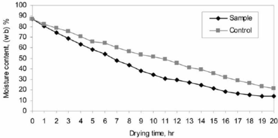
Fig. 13. Variations of moisture content with time for a typical experimental run during solar drying of pineapple.
