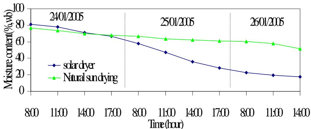
Fig. 16. Comparison of the moisture changes inside roof-integrated solar dryer and open sun drying during drying of chilli
