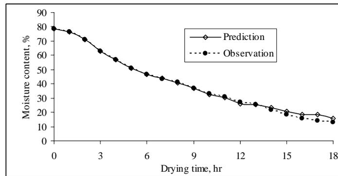
Fig. 25. Variation of predicted moisture content and observed moisture content of jackfruit leather with drying time
