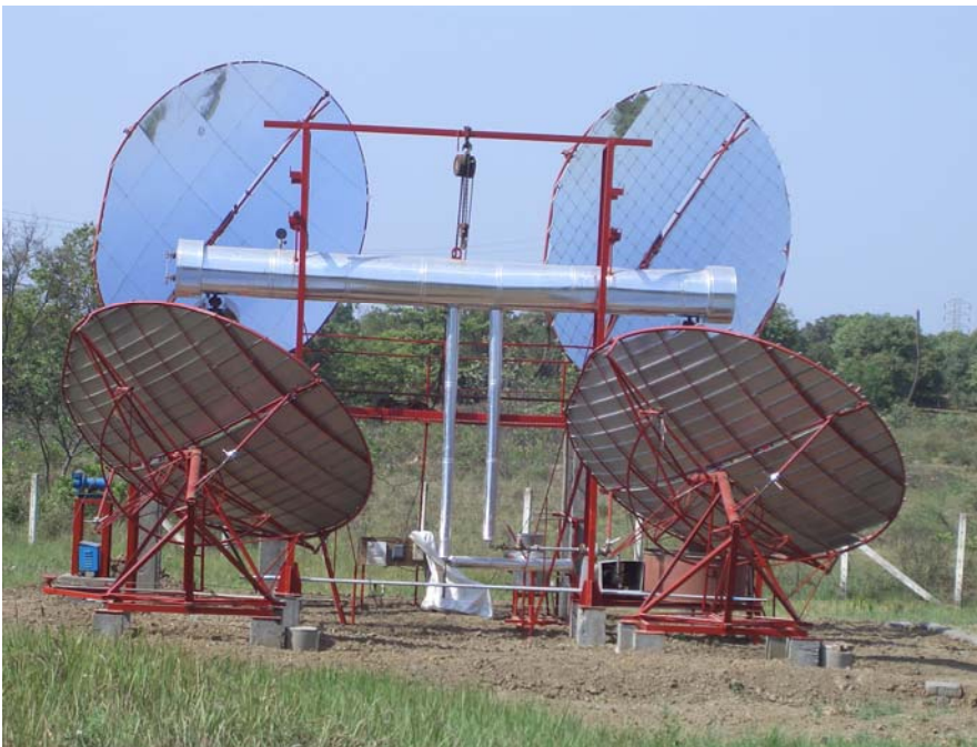
Fig. 3: Pilot plant for testing solar thermal energy for solar food processing, India 2005, Gadhia Solar
