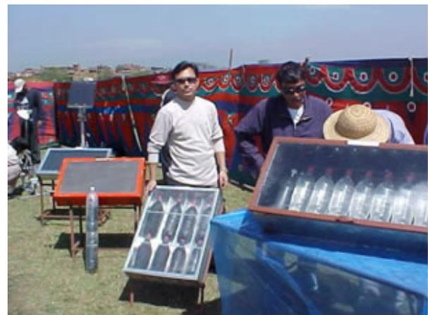
**Fig.3 Water Pasteurizers - different types by FoST**
