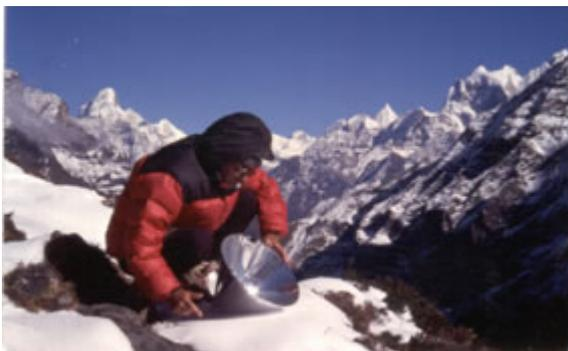
**Fig.4 Solar Backpack “Trekking” Cooker (made by FAST) preparing food or melting snow for drinking**
