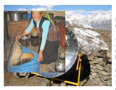
Parabolic Solar cooker and Heat-retaining basket used in mountain villages
