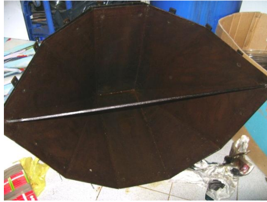
Fig. 9 – Bar welded to the internal piece of the mold
