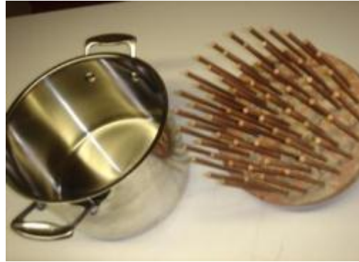
Figure 2. Stainless-steel 7-6-liter stockpot and finned underside of solid-copper hot-plate that together form a sealed container for molten salt
