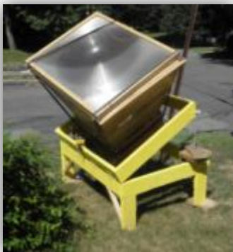
Figure 4 Three-degree-of-freedom frame built to test the performance of a plastic-sheet fresnel lens, which is on top, facing toward us. The lens and its support and the attached hot-plate and storage pot all swing on bearings, one of which is visible on the left side of the sloping frame. The basic, lower, frame is level and aligned accurately north (towards us) and south. The frame is adjusted to the sun's path at this latitude (42.3 degrees N) and time of year. The lens assembly has bicycle-inner-tube springs pulling it toward the afternoon position. The assembly is restrained by a clock movement so that it is aligned with the sun's position from the morning whether or not there are clouds.
