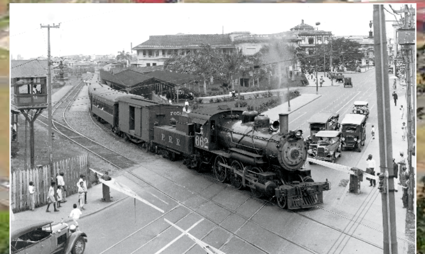
Partners in trade: The Port of Balboa and the Panama Canal Railway are adjacent to each other on the Pacific side of the canal. The Miraflores Locks are visible in the distance at upper right. Inset: Mogul-type locomotives were the principal freight and passenger power from the days of the canal's construction until the end of steam. Here, 2-6-0 No. 662 leaves Panama City in June 1930. Steam-era image: James H. Harrison collection
