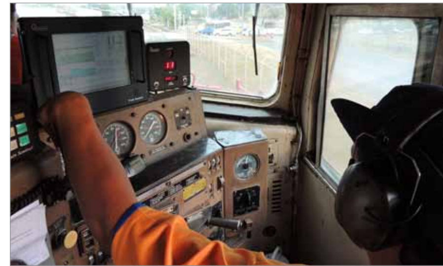
The morning commuter train leaves Balboa, bound for Colón, with engineer Omar Sanchez at the throttle. Note the positive train control monitor atop the control stand.
